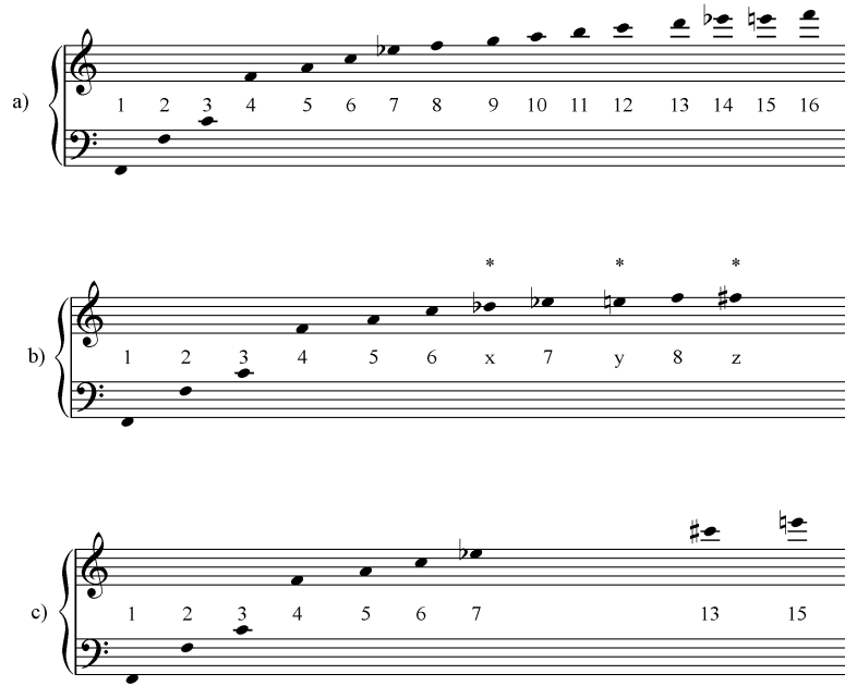
Figure 1: A comparison between a) an ideal harmonic series, b) the partials in a Rhodes sound, and c) the partials in a DX7 sound. Pitches marked with an asterisk (*) are inharmonic. Representation of pitches is approximate; the actual harmonic series does not adhere to the twelve-tone equal temperament implied by staff notation.
